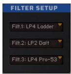
You can set up three filters here choosing from 30 different types. Click on the drop-down lists and select the filter type you wish for the three available slots.
