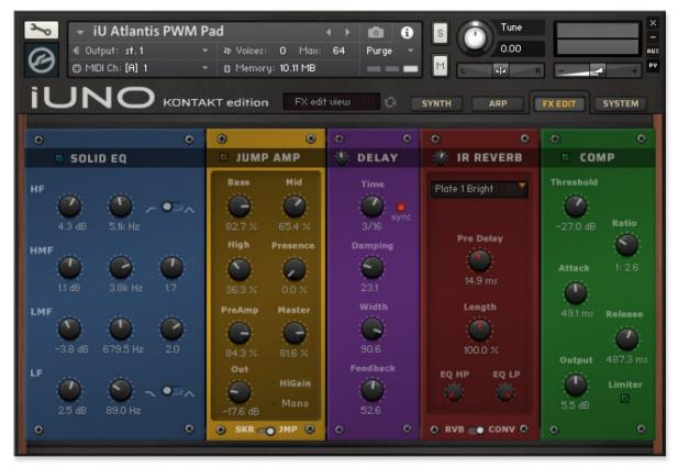
The **Solid EQ** is modelled on high quality analogue circuitry. It is a 4-band parametric EQ and offers the choice of bell or shelf style control of the low and high frequency bands.
