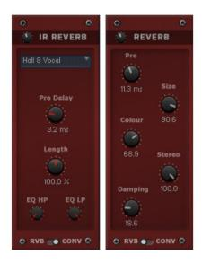
**Reverb** simulates the natural reverberation that occurs when a sound source is placed in an acoustic environment, thus adding a feeling of spaciousness to the sound.
