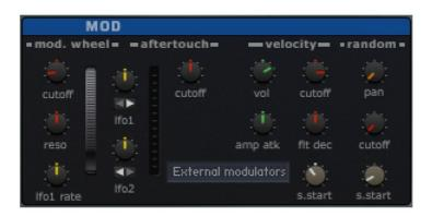
**Mod wheel** has five destinations: cutoff, resonance, LFO1 rate, LFO1 and LFO2 intensity.
