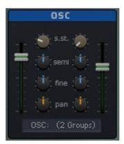
OSC volume: adjusts the group volume. This controller can be automated. Sample start offset: adjusts the sample start offset. Semi tune: transpose the OSC in semitune (+/- 12 st.) Fine tune: fine tune the OSC in one cent steps (+/- 100 cents) Pan: set the panorama of the OSC
